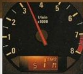
Shifting gears without the clutch thanks to BMW's Sequential M Gearbox (SMG).
