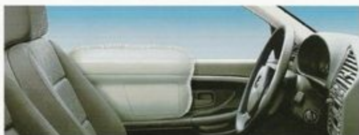
Side airbags for the driver and front passenger are standard on the M3.
