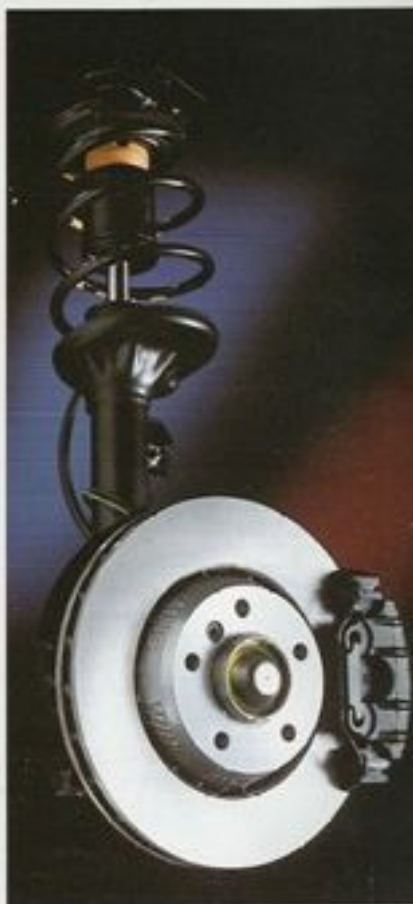
Compound discs with radial anti-friction bearings reduce fading on the high-performance brake system to an absolute minimum.
